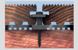
A predetermined breaking point that permits a flexible clamping range of 6 mm, enables alignment to various groove wall thicknesses. About 15 - 20 pieces are needed per m<sup>2</sup>, depending on board width.
