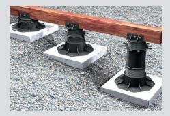
With the decking pedestals FTA-UF the easy and continuous height adjustment is done by simply turning to the right or left (even once installed). The adjustable pedestals provide secure support for the entire structure by adjusting the support rail for gradients which can easily be achieved. You will need approximately 3.5 - 5 decking pads per square meter.
