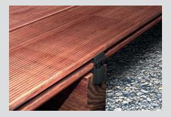
The start and end fixation FTA-ISW/ -ISA Start ensures invisible and clean fastening of grooved boards at the start and end of the completed decking. For all boards with central grooves of 4 mm or wider (mind. 9 mm deep).
