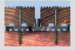
Furthermore, it guarantees spaces between the boards and support rails required for good ventilation. This ensures that any waterlogging that may have occurred can dry out. About 15 – 20 pieces are needed per m<sup>2</sup>, depending on board width.
